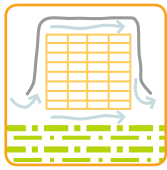
Ventilation under presenning
