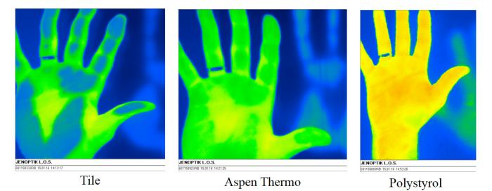
Figure 9. IR-temperature image of a human hand having touched for 10 seconds a tile, a thermally modified aspen board and a polystyrol board for 10 seconds at 23°C room temperature
