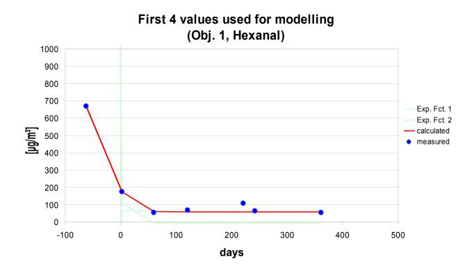
Figure 19. Modelled and experimental hexanal values
