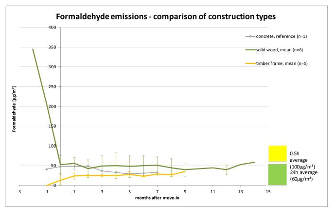
Figure 15. Formaldehyde emissions - comparison of construction sites
