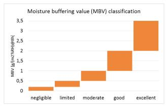
Figure 4. Moisture buffering value classes according to the NORDTEST method (5).
