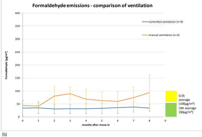
Figure 16. TVOC (a) and formaldehyde (b) emissions, mean values, comparison of controlled ventilation and manual venting
