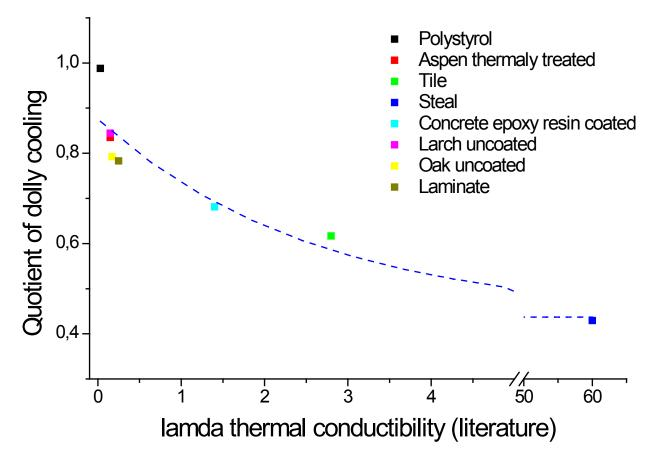
Figure 10. Quotient of dolly cooling after having touched different materials for 20 seconds
