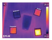
Figure 6. Pseudo colour image of the surface temperature on wood surfaces measured using thermal imaging
