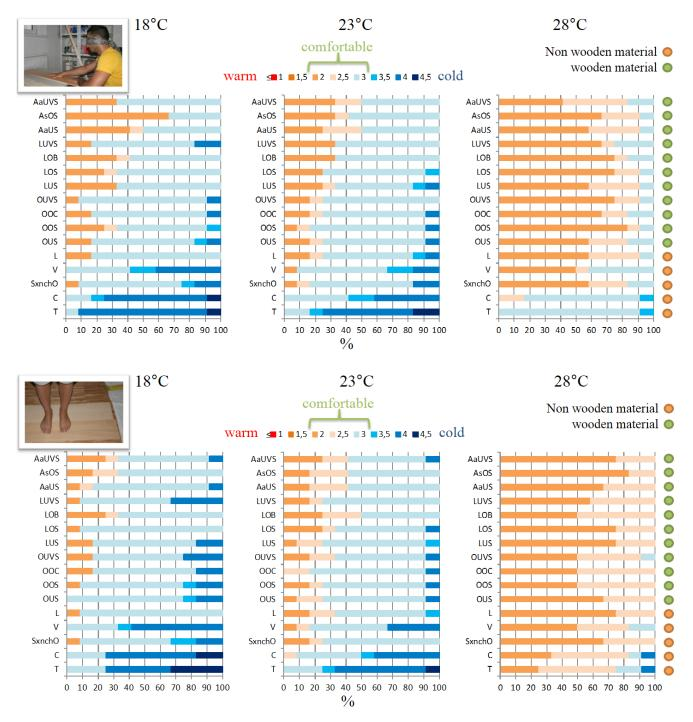
Figure 8. Temperature sensation with bar hand (top) and with bar feet (bottom) at material temperatures of 18°C, 23°C and 28°C
