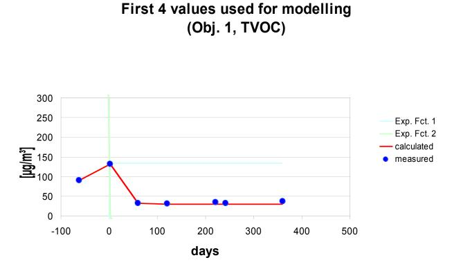
Figure 20. Modelled and experimental TVOC values
