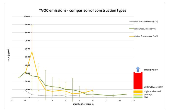
Figure 14. TVOC emissions – comparison of construction sites
