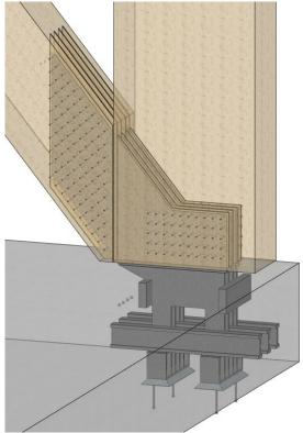
Figure 9: Connection at the foundation in each corner.
