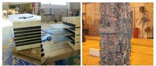
*Figure 11*: Sealed slots and gaps using intumescent fire strips.
