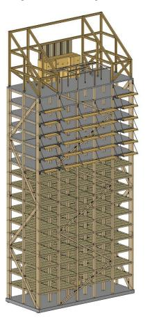
Figure 4: Structural system
