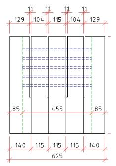
*Figure 8*: *Typical cross-section build-up with slotted-in steel plates and dowels.*
